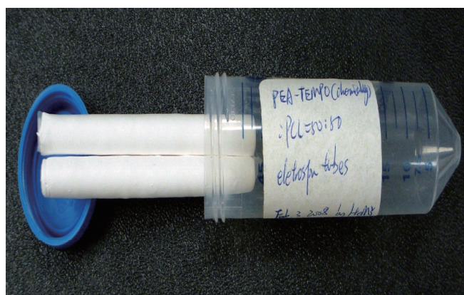
Fig. 24: Electrospun NOD-eluting Phe-based PEA tubular fibrous graft.
