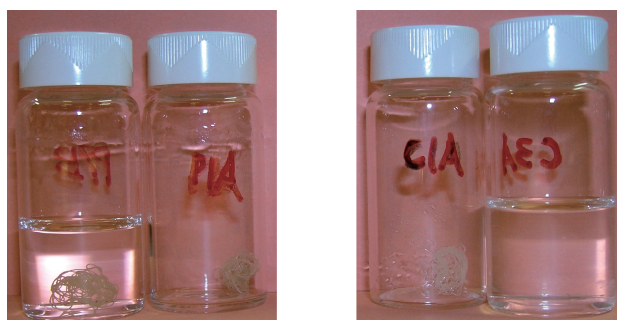
Fig. 6: In vitro enzyme hydrolysis of Phe-based PEA melt spun fibers at \alpha -chymotryps enzyme concentration of 0.1 mg/ml in 10 ml of PBS buffer. Left 2 bottles: in pure PBS for 1 (far left) and 2 days. Right 2 bottles: in enzyme/PBS solution for 1 and 2 (far right) days. No visible trace of AA-PEA fibers could be found at the end of the 2 days immersion in enzyme/PBS solution (far right).
