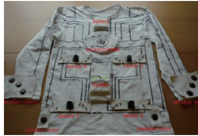
Fig. 6: A smart clothing system for obstacle avoidance [30]
