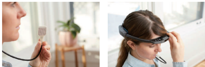
Fig. 14: Tongue array and wearing effect of BrainPort [36]
