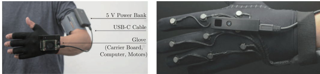
Fig. 13: Unfolding space glove wearing effect and detail picture [35]
