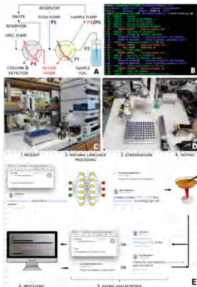
Figure 2. (A) Schematic of the flow path for the sampling sequence used with the N9 robotic platform. The six parameters (P1-P6) are color coded to illustrate the effect they have on the sampling sequence. The yellow shade highlights the arm valve, and the grey shade the HPLC valve. (B) Example of logging messages from ChemOS. (C) Side and (D) top view of the robotic hardware. Lower panels: Results from the autonomous calibration of an HPLC setup maximizing the magnitude of the response. (E) Representation of the ChemOS pipeline while screening the Tequila Sunrise space [25].
