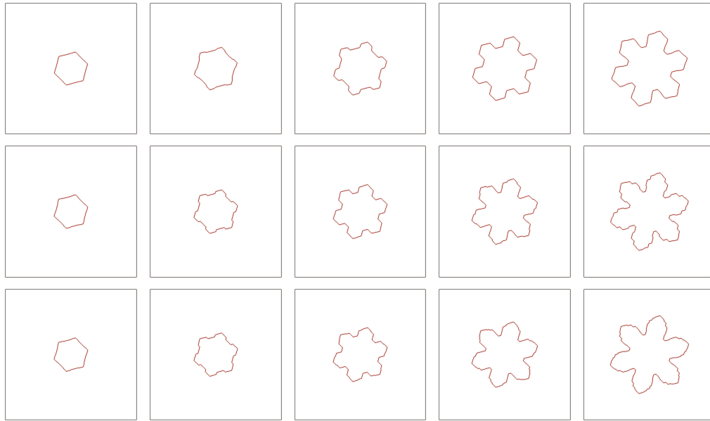
Figure 18: (PFEM, \text{ANI}_2 , \vartheta=1 , \alpha=5\times 10^{-4} , \rho=0.01 , u_D=-\frac{1}{2} , \Omega=(-2,2)^2 ) Snapshots of the solution at times t=0.3, 0.4, 0.5, 0.6, 0.7 . From top to bottom \tau=10^{-k} , k=2, \dots, 4 . [These computations took 1, 9 seconds and 87 seconds, respectively.]
