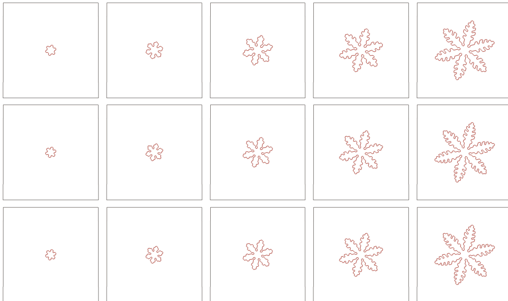
Figure 19: (PFEM, \text{ANI}_2 , \vartheta=0 , \alpha=10^{-5} , \rho=1.42\times 10^{-3} , u_D=-0.04 , \Omega=(-4,4)^2 ) Snapshots of the solution at times t=5, 10, 20, 30, 40 . From top to bottom \tau=10^{-k} , k=1, \dots, 3 . [These computations took 6, 124 and 781 minutes, respectively.]
