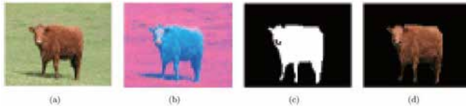
Figure 3: An example using MSRG to detect and extract. (a) The original image; (b) the segmented image; (c) the binary image; (d) the salient object image.
